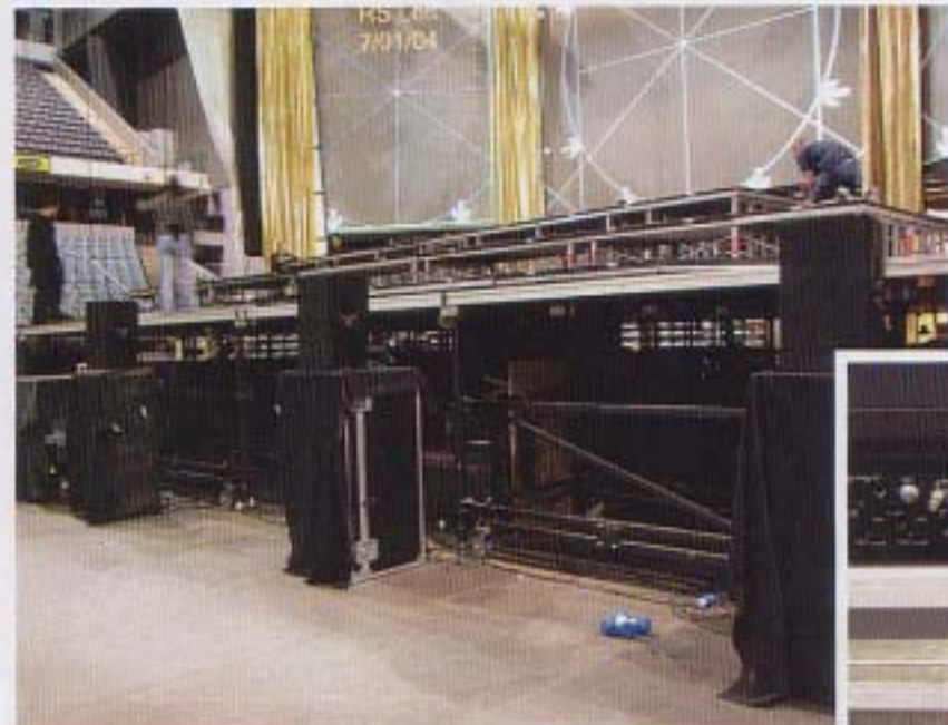
Wide-coverage loudspeakers on road cases for front fill, and (right) clean I/O at the house console.
