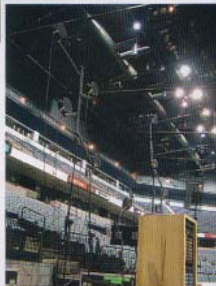
Now that's some serious RF! Antenna jungle above, stacks of AKG wireless receivers below in the wood case.
