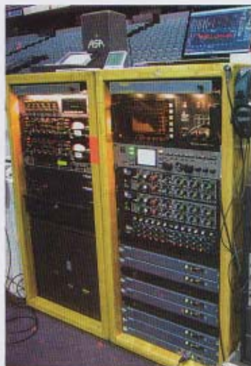
The two racks at front of house, topped by laptop with SMAART. Also note one of the first sightings of the new TC Electronic EQ Station, in the right rack under the dbx RTA-1.
